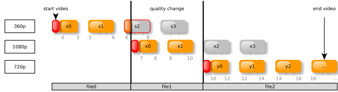
Fig. 2. Example of assembling a video stream; three different quality switches occur during video play-out and reassemble video files for our analysis.
